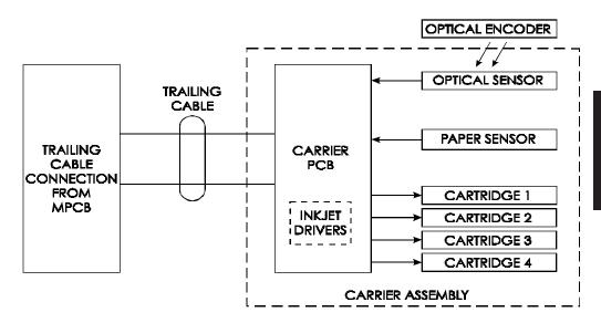
Figure 2-10. Carrier Assembly Circuits.
